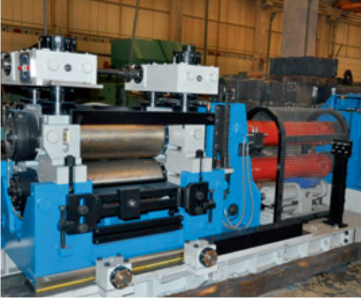
HADDE TEZGAHI ÖN GERİLMELİ FINISH GRUP (Max. 345 - Min.275 mm) (Roll Stands Housingless Type)
